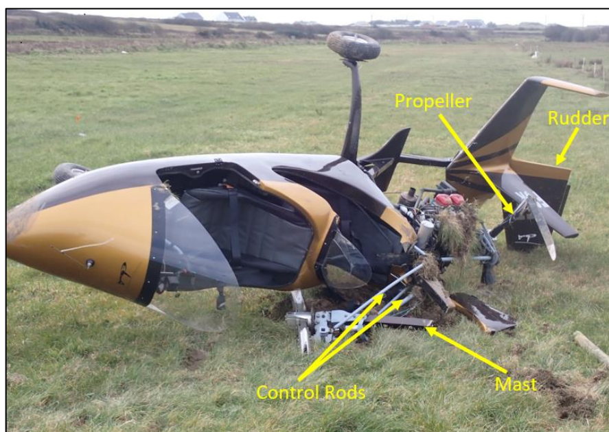
Photo No. 3: Damage to control rods, mast, propeller and rudder
